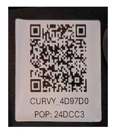
You can find a QR code sticker like this attached on your device. This QR code sticker also locates the position of the touch sensor which helps in rebooting the device when you want to re-do the provisioning in case of Wi-Fi password change or Wi-Fi network change if any in future. You just have to long press this sticker for
